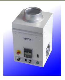
The dual asymmetric DAC 150 FV-K shown in the photograph works by spinning a high speed-mixing arm in one direction while the basket rotates in the opposite direction (thus, the name - Dual Asymmetric Centrifuge). This combination of forces in different planes enables incredibly fast mixing, and yet the precision construction of each machine gives it a balance that allows amazingly quiet operation
